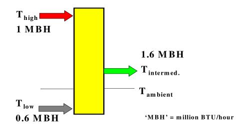
Figure 1. Trithermal Heat Activated Heat Pump/Chiller
