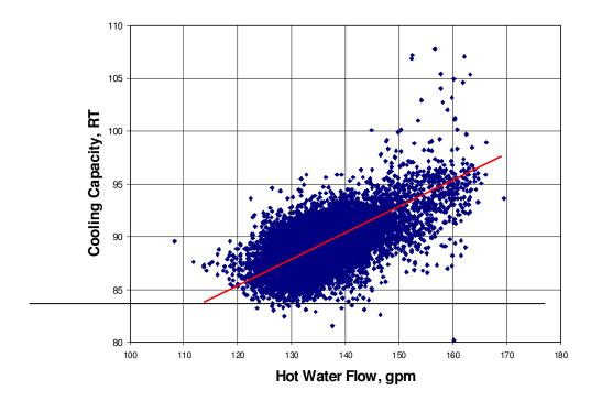
Figure 5. Water Flow Effect on HAHP/C Capacity
