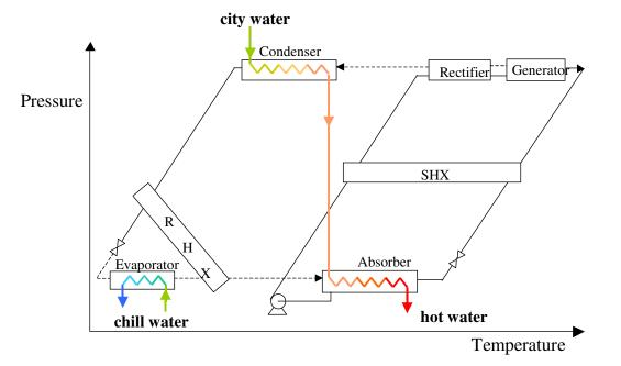
Figure 2. Thermodynamic Diagram of Ammonia Absorption HAHP/C
