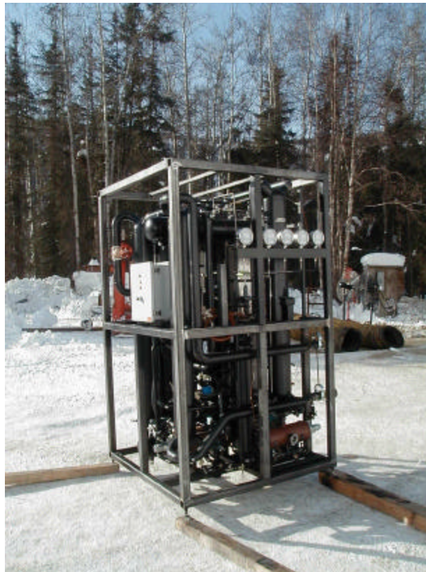
Fig. 3 Double lift ThermoChiller prior to installation
